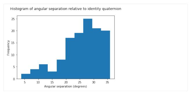
As a simple check, we can ensure that for the identity quaternion (1, 0, 0, 0), which performs a 0° rotation, the angles between the reference orientations and that quaternion are equal to the original angles of rotation of those quaternions (*i.e.* how much those orientations were already rotated relative to the identity).
