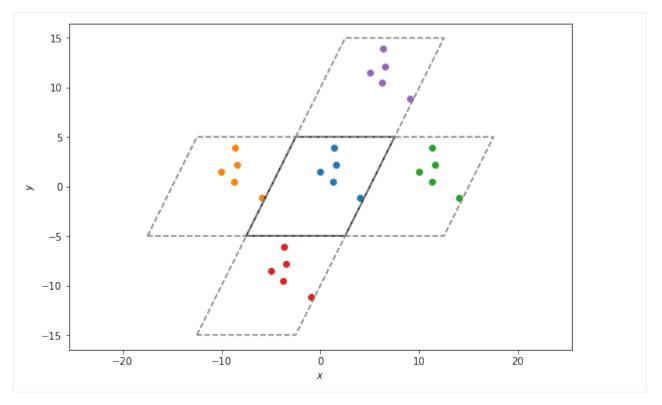
Box wrapping takes points in the periodic images of a box, and brings them back into the original box. In this context, that means that if we apply wrap to each of the sets of particles plotted above, they should all overlap.
