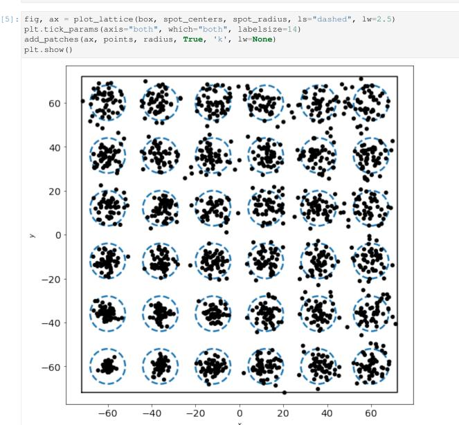
We see that the density decreases as we move up and to the right. In order to compute the actual densities, we can leverage the LocalDensity class. The class allows you to specify a set of query points around which the number of other points is computed. These other points can, but need not be, distinct from the query points. In our case, we want to use the blue regions as our query points with the small black dots as our data points.
