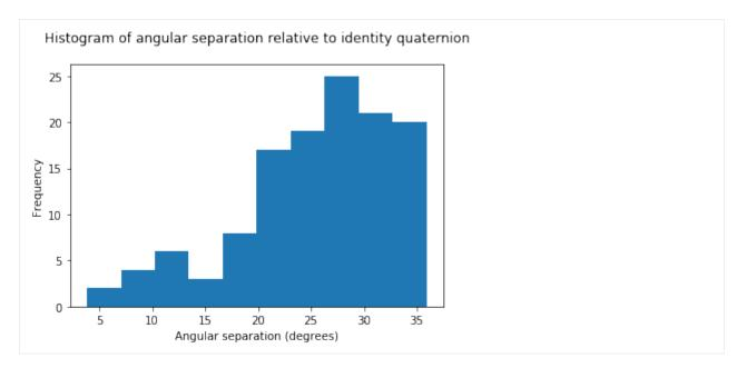
As a simple check, we can ensure that for the identity quaternion (1,0,0,0), which performs a  $0^{\circ}$  rotation, the angles between the reference orientations and that quaternion are equal to the original angles of rotation of those quaternions (*i.e.* how much those orientations were already rotated relative to the identity).
