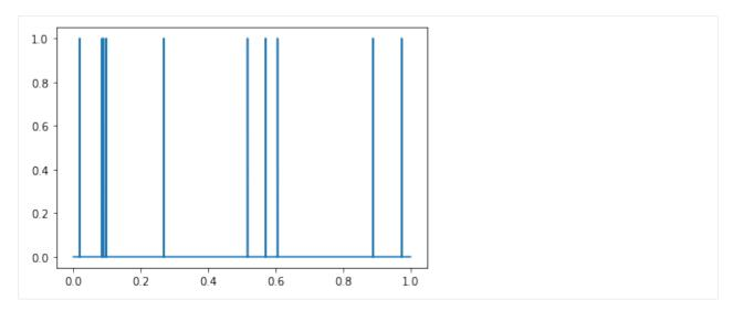
However, delta functions can be cumbersome to work with, so we might instead want to smooth out these particles. One option is to instead represent particles as Gaussians centered at the location of the points. In that case, the total particle density at any point in the interval [0,1] represented above would be based on the sum of the densities of those Gaussians at those points.
