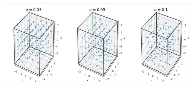
If we recompute the Steinhardt OP for each of these data sets, we see that adding noise has the effect of smoothing the order parameter such that the peak we observed for the perfect crystal is no longer observable.
