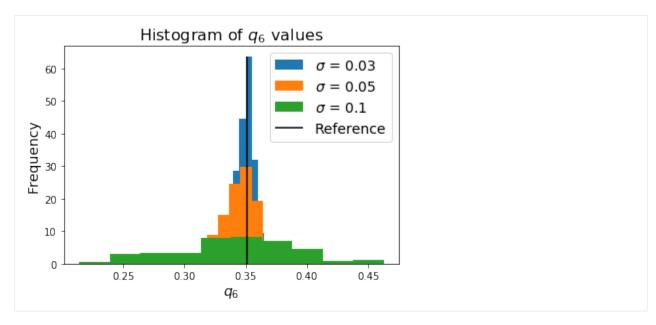
This type of identification process is what the LocalDescriptors data outputs may be used for. In the case of Steinhardt OPs, it provides a simple fingerprint for comparing thermalized systems to a known ideal structure to measure their similarity.
