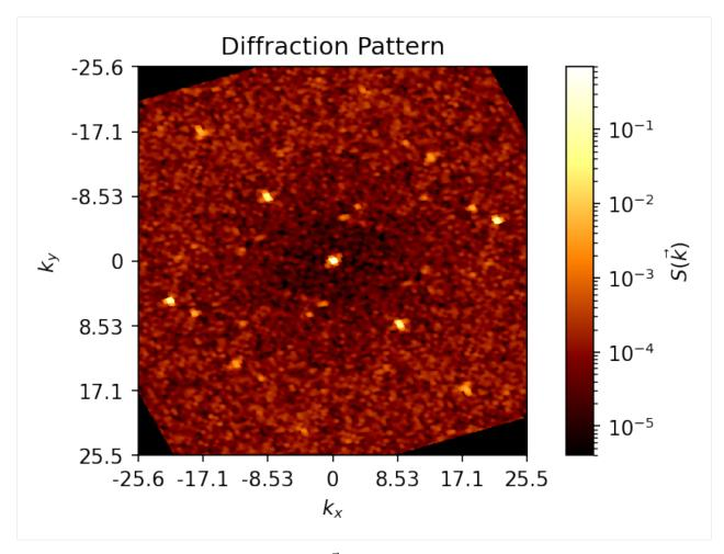
The DiffractionPattern object also provides  $\vec{k}$  vectors in the original 3D space and the magnitudes of  $k_x$  and  $k_y$  in the 2D projection along the view axis.
