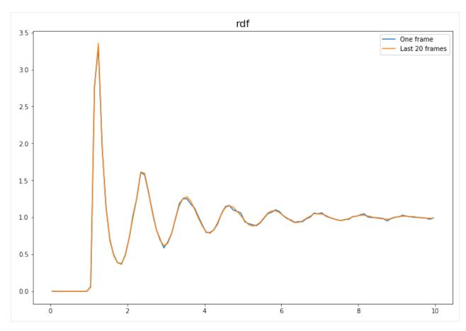
The difference between accumulate (which should be called on a series of frames) and compute (meant for a single frame) is more striking for smaller bin sizes, which are statistically noisier.
