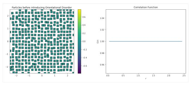
Now we will generate random angles from  $-\frac{\pi}{4}$  to  $\frac{\pi}{4}$ , which orients our squares randomly. The four-fold symmetry of the squares means that the space of unique angles is restricted to a range of  $\frac{\pi}{2}$ . Again, we compute a complex value for each particle,  $s=e^{4i\theta}$ .
