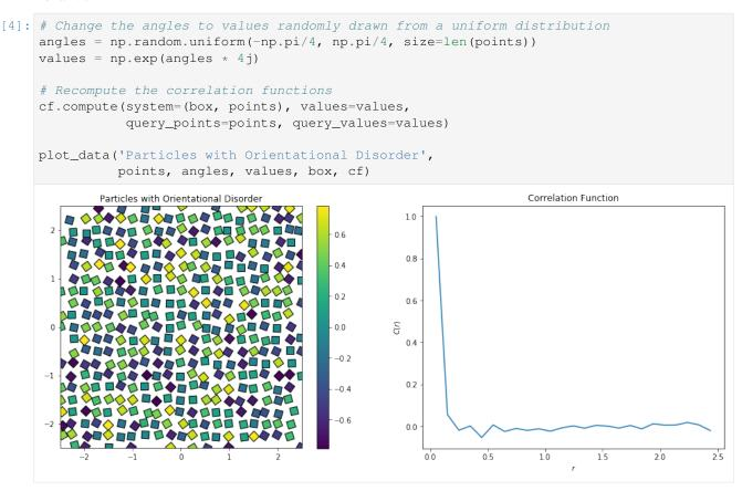
The plot below shows what happens when we intentionally introduce a correlation length by adding a spatial pattern to the particle orientations. At short distances, the correlation is very high. As r increases, the oppositely-aligned part of the pattern some distance away causes the correlation to drop.
