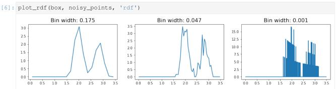
In this RDF, we see the same rough features as we saw with the perfect lattice. However, the signal is much noisier, and in fact we see that increasing the number of bins essentially leads to overfitting of the data. As a result, we have to be careful with how we choose to bin our data when constructing the RDF object.
