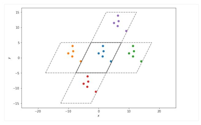
Box wrapping takes points in the periodic images of a box, and brings them back into the original box. In this context, that means that if we apply wrap to each of the sets of particles plotted above, they should all overlap.
