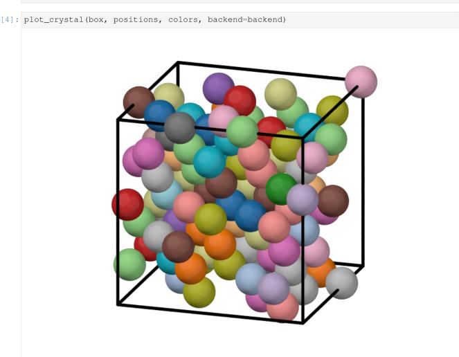
We make a Voronoi tesselation of the system and plot it in 3D. The Voronoi cells are approximately rhombic dodecahedra, which tesselate 3D space in a face-centered cubic lattice.
