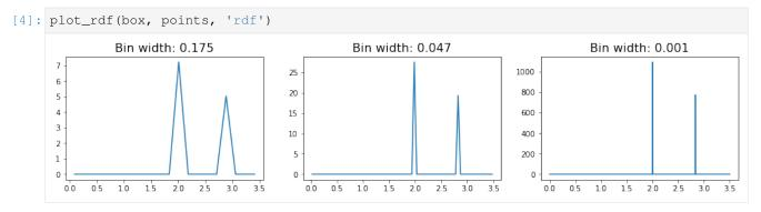
In these RDFs, we see two sharply defined peaks, with the first corresponding to the nearest neighbors on the lattice (which are all at a distance 2 from each other), and the second, smaller peak caused by the particles on the diagonal (which sit at distance  $\sqrt{2^2 + 2^2} \approx 2.83$ .
